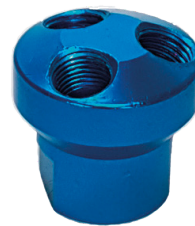
3/8 bsp female inlet 3 x 1/4 bsp outlets
